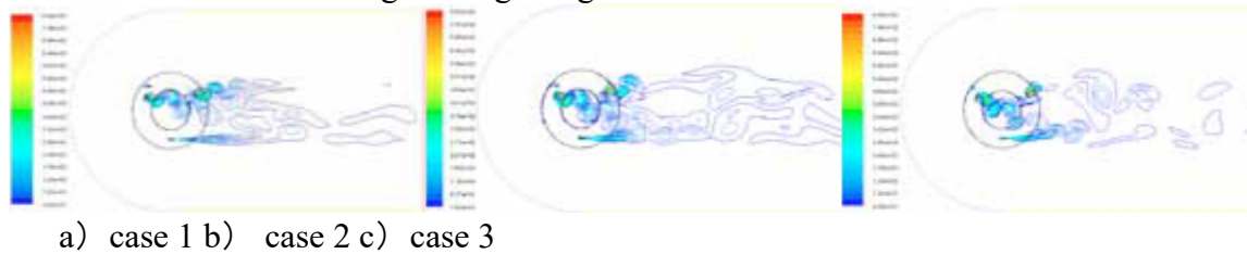
Fig.7. distribution of turbulent kinetic energy ( m^2/s^2 )
